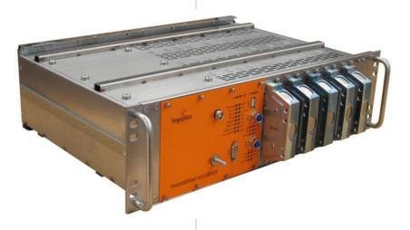
The Crash Protected Memory Module (CPMM) fulfils world standards such as the European EEIG 97E461.3, the British GM/RT2472 and IEEE1482.1 standards for the Juridical Recording Unit (JRU).
